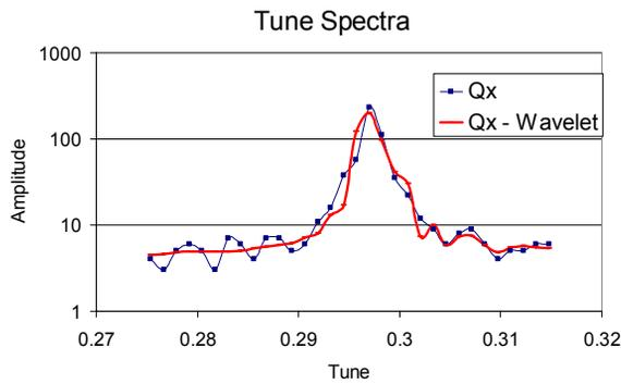
Figure 4: Comparison of raw and filtered tune spectrum.
