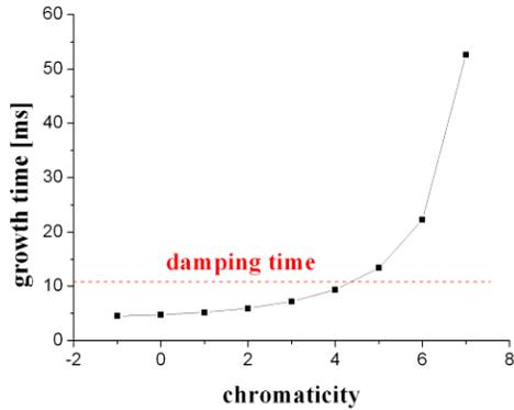
Figure 3: Growth time of resistive wall instability as a function of the vertical chromaticity for coupled bunch mode 851. The radiation damping time is 10.5 ms.
