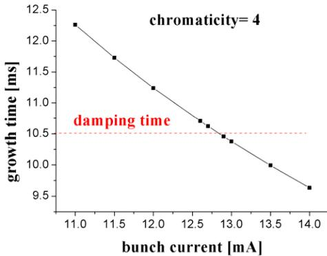
Figure 4: Calculated growth time of  $\ell= 1$  single bunch head-tail mode. The radiation damping time is 10.5 ms.
