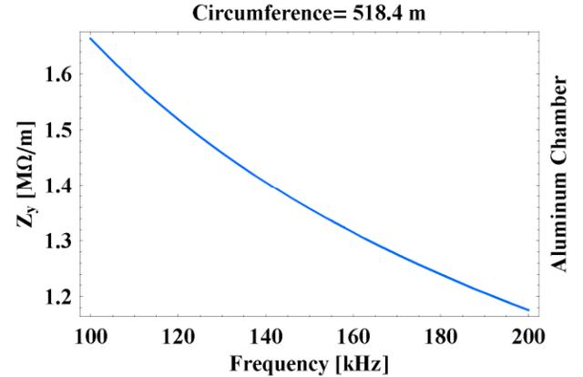
Figure 2: The vertical resistive wall impedance of TPS beam pipe without any insertion device. The frequency of the lowest betatron sideband is around 162 kHz.
