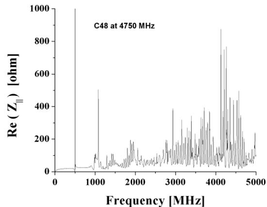
Figure 1: The longitudinal impedance of a CESR SC RF cavity module calculated by the 3-D code GdfidL.
