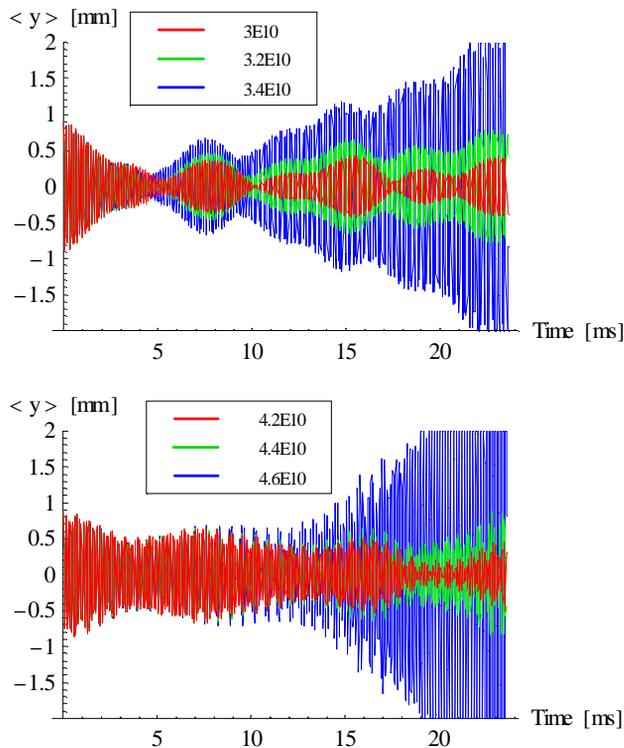
Figure 1: Evolution of the vertical centroid position vs. time (up to 1024 SPS turns, i.e.  $\sim 23$  ms): (upper) without linear coupling, (lower) with optimum linear coupling. In the legend the numbers refer to the number of protons per bunch.
