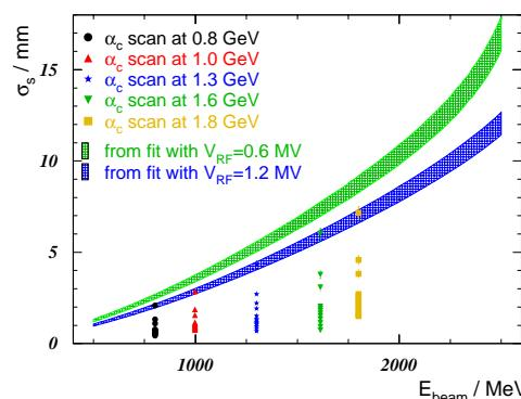
Figure 2: RMS Bunch length derived from measurements of  $f_s$  (see Fig. 1) as a function of beam energy. The hatched regions are error bands obtained by a full error Monte Carlo. The markers represent bunch lengths derived from synchrotron frequency measurements for different beam energies.
