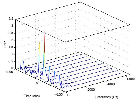
Figure 7: Lomb Normalised Periodograms of the bolometer signal during the evolution of a burst for a bunch current of 0.16 mA. The intensity maximum of the burst is also visible in the frequency spectrum.
