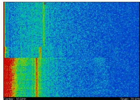
Figure 9: Spectrogram of the bolometer signal as a function of time (moves downward) during a “low  $\alpha_c$  squeeze” at a (constant) low bunch current. The steps in synchrotron frequency are clearly visible.
