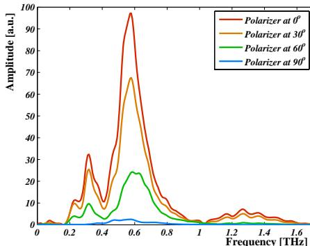
Figure 4: The FIR spectrum measured at a beam energy of 1.3 GeV ( $V_{RF} = 1.2$  MV,  $f_s = 7.1$  kHz) for different orientations of the polarising grid. The 0° position corresponds to a horizontal, the 90° to a vertical orientation.
