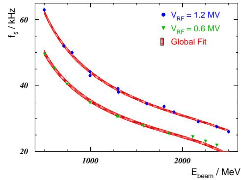
Figure 1: Measured synchrotron frequencies as a function of the beam energy for different total voltages in the RF cavities. The hatched areas denote the error bands of a global fit of the momentum compaction factor to the full dataset.
