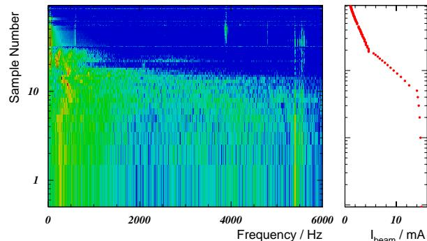
Figure 8: Evolution of the bolometer signals frequency spectrum with decreasing beam current (increasing sample number). The synchrotron frequency is 5.5 kHz.
