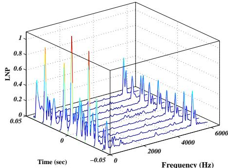
Figure 6: Lomb Normalised Periodograms of the bolometer signal during the evolution of a burst (at  $t = 0$ ). This dataset was recorded at a relatively high bunch current (0.47 mA) and at a beam energy of 1.3 GeV.
