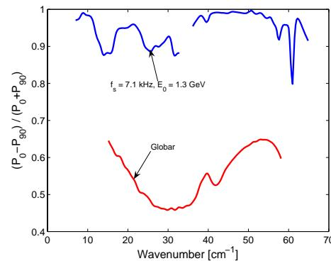
Figure 5: Degree of polarisation derived from the measurements shown in Fig. 4 and from a measurement with an internal source (Globar) as a function of frequency. The visible polarisation of the internal source indicates a residual polarisation of the detection system.
