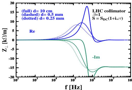
Figure 2: Transverse impedances for different wall thicknesses LHC collimator)
