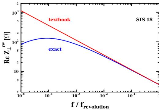
Figure 1: Comparison between exact (blue) and textbook result eq.(2), of the real part of the transverse resistive wall impedance (SIS18)
