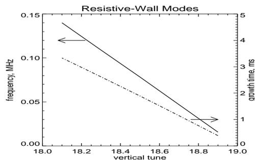
Figure 2: Frequency (full line) and growth times (chain line) for the resistive wall instability for SIS100 conditions.
