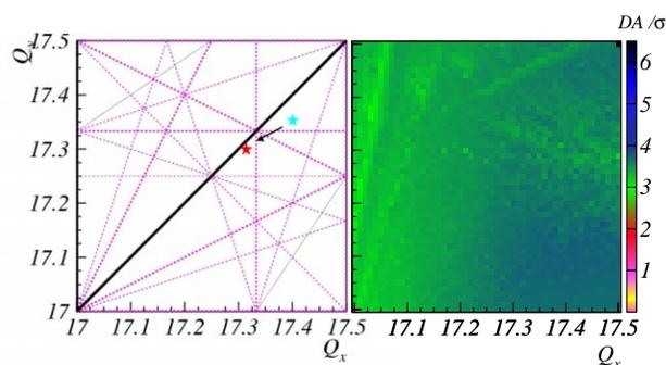
Figure 4: Left: WP2 before acceleration (blue star) and for slow extraction (red star). Right: Scan of DA at 1000 turns for  $I=640$  A.
