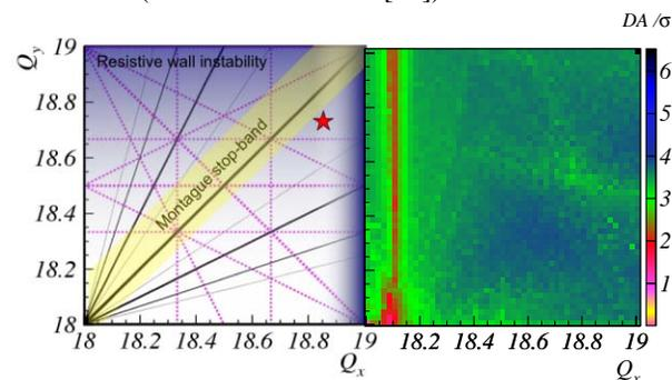
Figure 3: Left: Schematic of tune diagram, with red star marking the proposed working point (WP1). Right: scan of DA at 1000 turns over same tune area.
