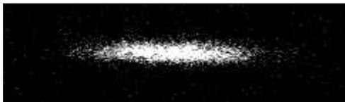
Figure 3: The measured beam profile by using newly installed mechanical shutter
