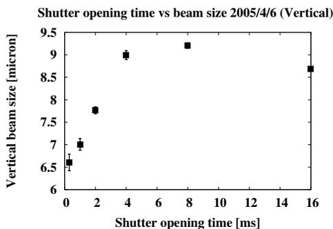
Figure 5: The shutter opening time vs vertical beam sizes
