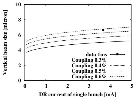
Figure 8: The comparison between the measured vertical beam size and calculation
