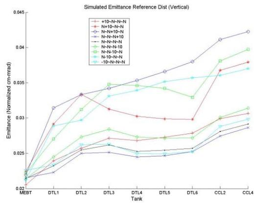
Figure 6. Simulated vertical emittance growth.
