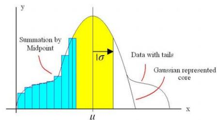
Figure 2. Pictorial representation of the area ratio method.
