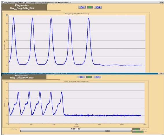
Figure 5:  $3.0 \times 10^{13}$  ppp (upper) and  $5.5 \times 10^{13}$  ppp (lower) are shown circulating in the ring shortly before extraction.
