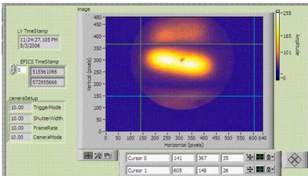
Figure 6: View screen picture of a fully painted proton beam on target with almost nominal beam size.
