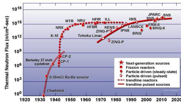
Figure 2: Neutron Source Development over the last 70 years for fission and spallation sources.
