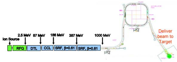
Figure 3: Schematic layout of the linac and the accumulator ring.
