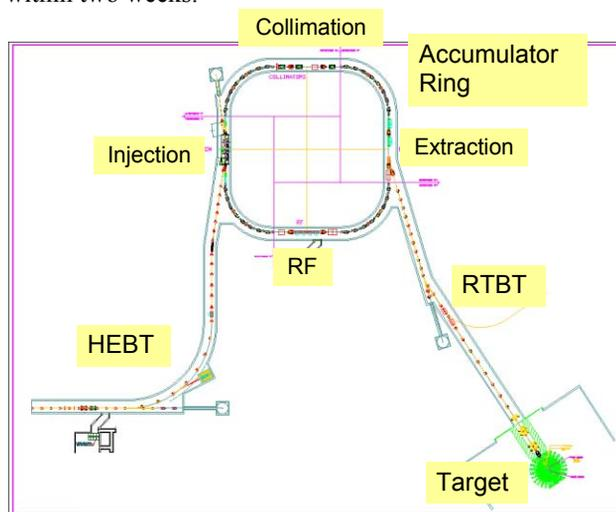
Figure 4: Layout of the accumulator ring and the associated beamlines.
