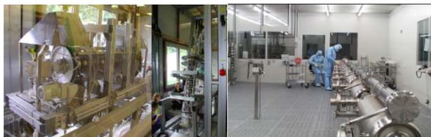
Figure 1: EP facility in TTF (left), Cavity String Assembly (right)
