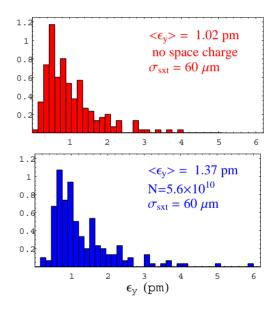
Figure 3: Frequency plot of equilibrium vertical emittance with and without space charge.
