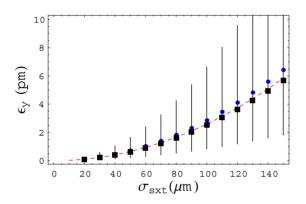
Figure 1: Equilibrium vertical emittance as a function of a random rms vertical displacement of the sextupoles. Boxes are the average values over the 5%-95% percentile range of the emittances found; the dots the average over the full range. Space charge not included.
