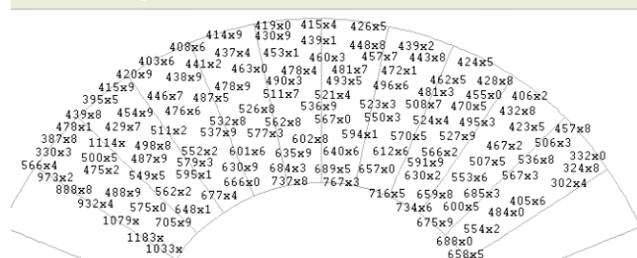
Figure 2. Current density in cross-section of conductor,  $kA/cm^2$ . The conductor is twisted counterclockwise.  $x$  used as decimal separator.
