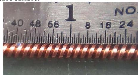
Figure 1: Scaled view on the undulator windings [2]. Wire with rectangular cross-section has dimensions 0.6×0.6 mm<sup>2</sup>, period  $\cong$  2.54 mm.
