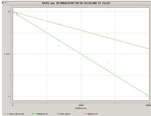
Figure 5: Transverse displacement of the beam along longitudinal distance. Lower curve corresponds to undulator filled with oil –the upper –to the undulator filled with ferrofluid.
