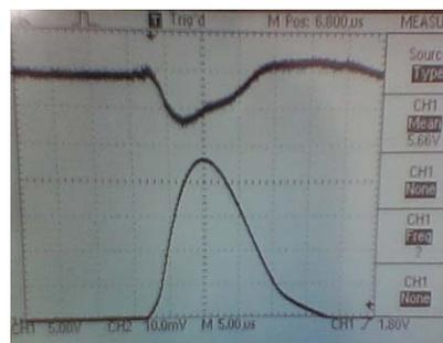
Figure 3: Shunt signal, low curve. Voltage-upper curve. Shunt calibration -100A/V.
