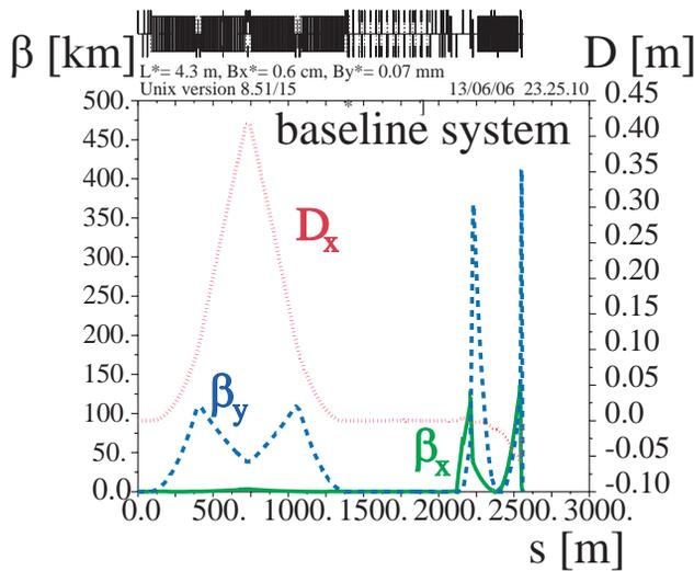
Figure 3: Optics of the CLIC baseline 3-TeV beam-delivery system with 2-km long collimation section, for  $\beta_x^* = 6$  mm,  $\beta_y^* = 70$   $\mu$ m.
