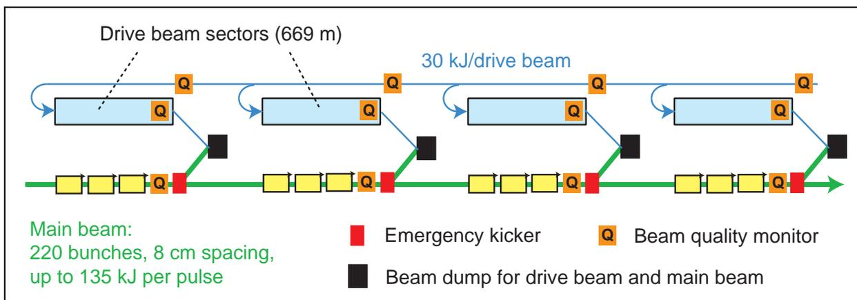
Figure 2: Emergency kickers for active machine protection and shared beam dumps along the CLIC main linac.
