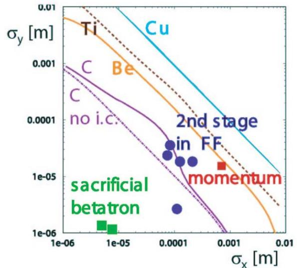
Figure 1: CLIC damage threshold diagram: minimum horizontal and vertical rms spot sizes in case of beam impact on various materials (for carbon calculations with and without the effect of image currents are shown) [1]. The nominal beam sizes at various collimator positions in the present CLIC collimation system and final focus are also indicated by the plotting symbols [3].
