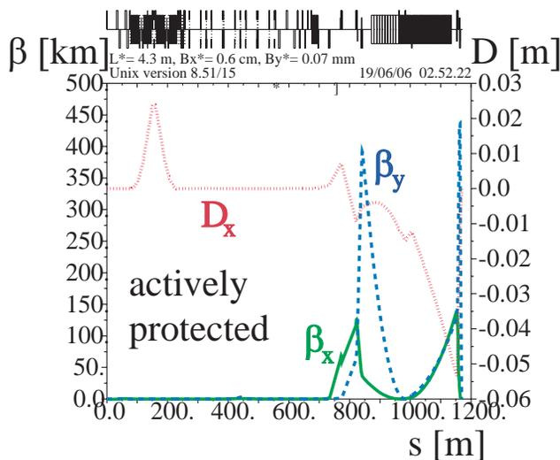
Figure 4: Optics of the proposed shorter 3-TeV beam-delivery system with 0.5-km long collimation section, for  $\beta_x^* = 6$  mm,  $\beta_y^* = 70$   $\mu$ m.
