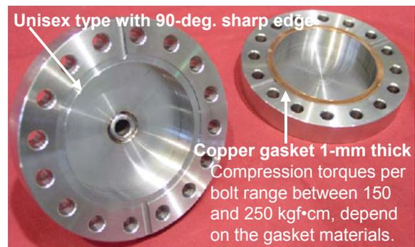
Figure 1: A photograph of a 130-mm diameter prototype flange (MO-unisex flange).
