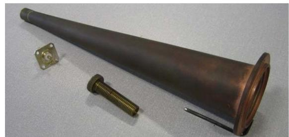
Figure 1: Launch cone, wire tensioner and N-type connector.
