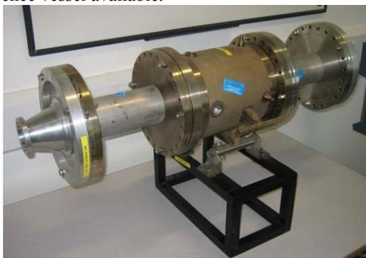
Figure 3: Cavity BPM, Device under test.
