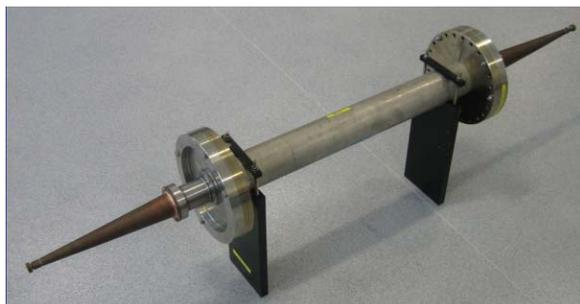
Figure 4: Reference vessel with launch cones connected.
