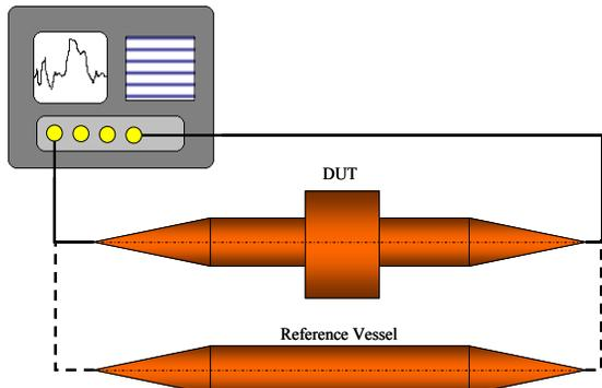
Figure 2: Schematic of the wire test apparatus.
