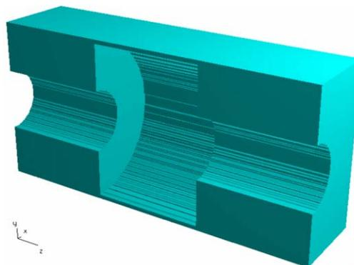
Figure 6: Mafiac model of Cavity BPM.
