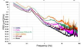
Figure 1: Average PSDs, in the vertical direction, of several sites, including a reference site, Moxa
