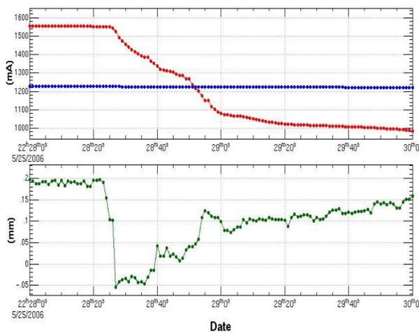
Figure 3: An example of a sudden horizontal orbit change observed at the crab cavity location in the HER (bottom). The LER and HER beam currents are plotted in the top figure.
