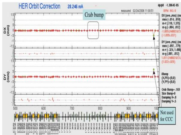
Figure 8: Deviation from the gold orbit in the Nikko crab section is shown when both CCC and crab feedback were on.
