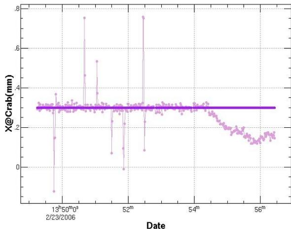
Figure 6: Beam orbit at the crab cavity in the HER. Dots are the measured orbit and the solid line is the target orbit. Spikes indicate the COD generated by an intentional single kick.
