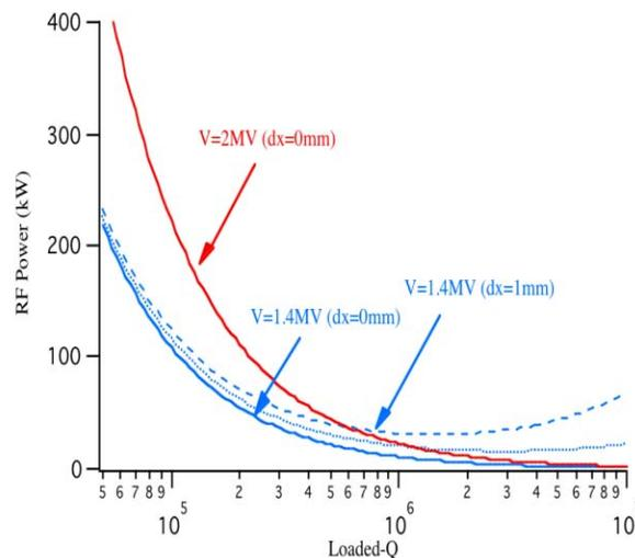
Figure 2: Required RF power vs. Loaded-Q.
