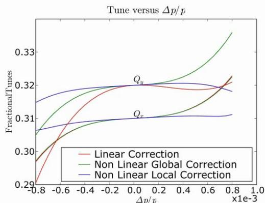
Figure 3: Horizontal and vertical chromaticity for Beam 1 after several correction options.
