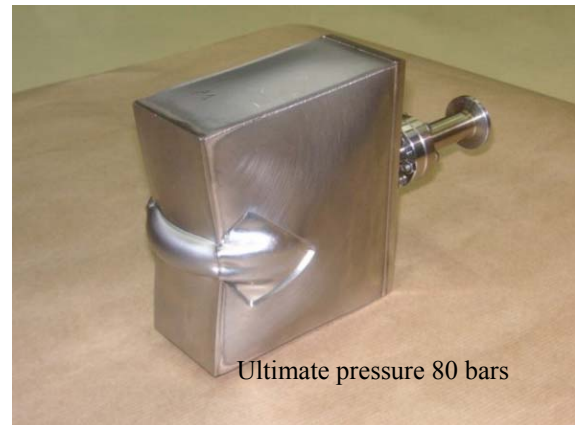
Figure 6: Deformation of the thin window after the ultimate pressure test, stopped at 80 \text{ bars} .
