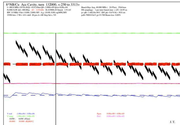
Fig 2b: As Fig. 2a but after adaptation for 132000 turns (about 11 s): nearly constant RF power. Bunch positions now shifted as already shown in [2], energy deviation from equilibrium ±0.4 MeV. Cavity tuning drifts from half-detuning at -2.76 kHz to -4.32 kHz.
