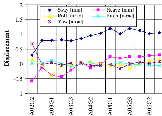
Figure 4: Post-construction survey results. Data shown for girders selected for priority realignment.
