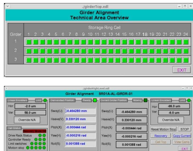
Figure 3: Operator panel indicating ready status for each girder (top) and panel for girder positioning (bottom).
