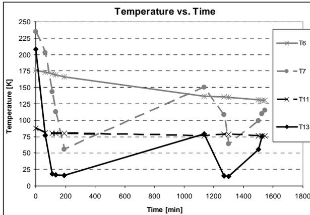
Figure 5: Results after pre-cooling with LN2 (T6: beam tube; T7: c/w-transition; T11: LHe supply tube; T13: exhaust gas).
