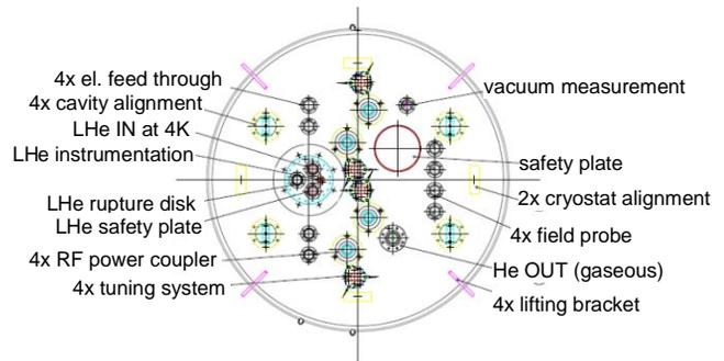
Figure 4: Instrumentation and Measurement Equipment on the top of the cryostat.
