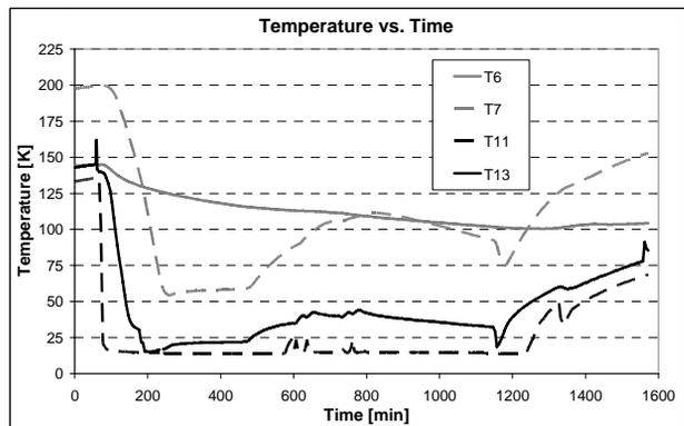
Figure 6: Results after pre-pumping (T6: beam tube; T7: c/w-transition; T11: LHe supply tube; T13: exhaust gas).
