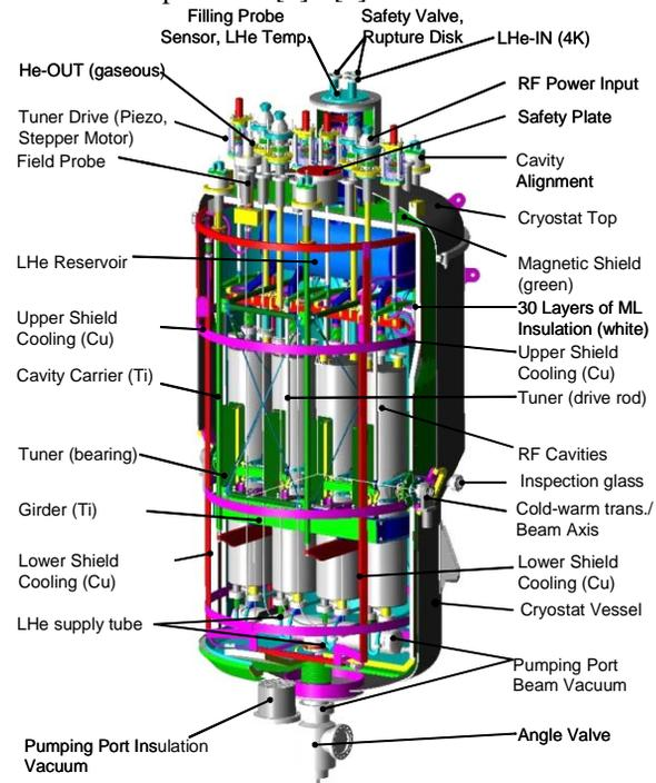
Figure 1: Cryostat Design (Cu sheets of the shield cooling system are partly removed).
