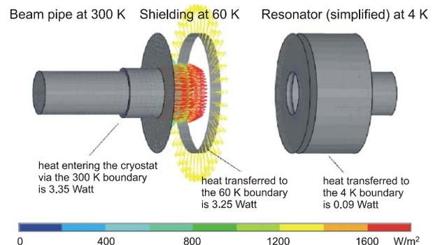
Figure 2: Numerical calculation of the heat transfer for the cold-warm transition at the beam tubes [6].
