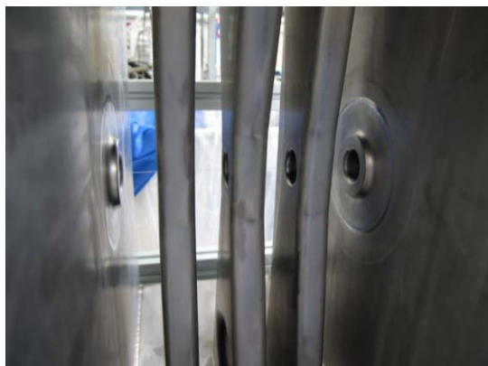
Figure 1: Inner view of the full Nb prototype of the \beta=0.12 Ladder resonator, after completion of the construction procedure.
