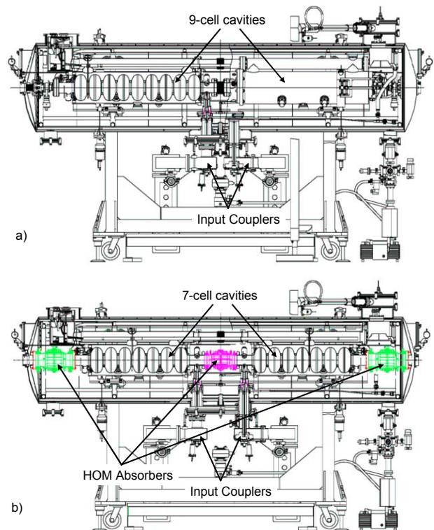
Figure 5. a)Original and b)Modified Cavity/Cryomodule.
