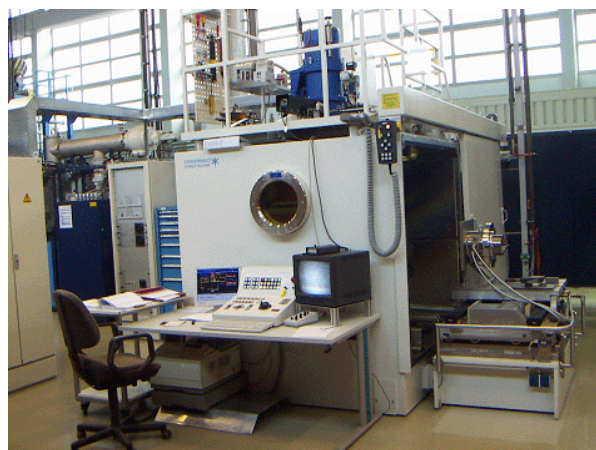
Figure 6: New electron beam welding machine.
