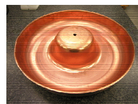
Copper end cup prototype after spinning
