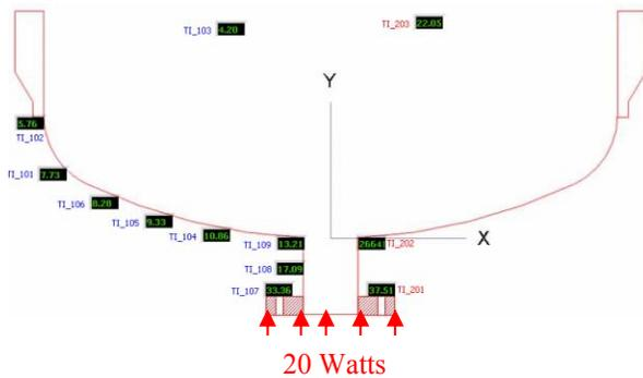
Figure 5: Statement of the temperatures in Kelvin along the cavity bottom for 20 W of heating. One has to consider the values indicated for the blue tags.
