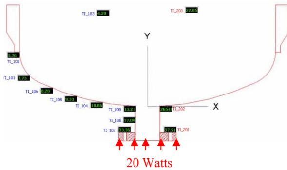
Figure 5: Statement of the temperatures in Kelvin along the cavity bottom for 20 W of heating. One has to consider the values indicated for the blue tags.
