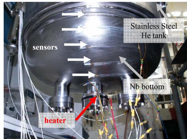
Figure 3: Heater set-up on the cavity bottom.
