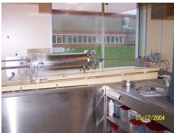
Figure 1: Beta 0.07 QWR inside the clean room during the High Pressure Rinsing process.
