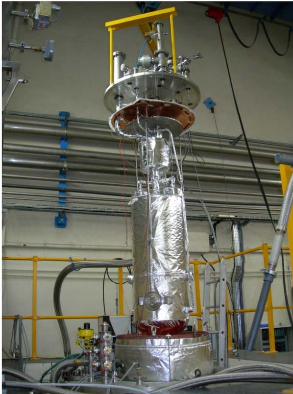
Figure 2: Beta 0.12 QWR before cold test.
