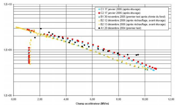
Figure 2: All the RF tests results of the beta 0.07 QWR since 2005.
