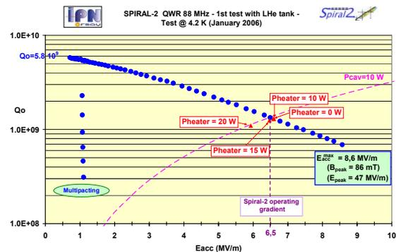
Figure 4: RF results at 4.2 K.  $Q_0$  measurements with the heater power: red triangles.
