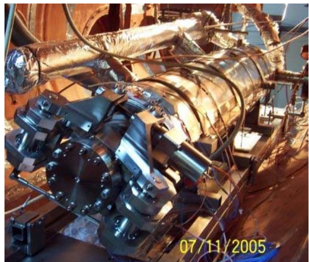
Figure 1: TTF 9-cell cavity with PTS in CryHoLab.
