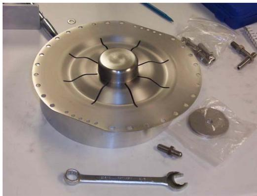
Figure 6. Compensation puck assembled and welded to the tuning plate.
