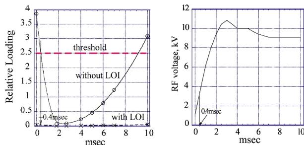
Figure 4: (left) relative beam loading of a second harmonic cavity with and without LOI. (right) required second harmonic voltage per cavity gap.
