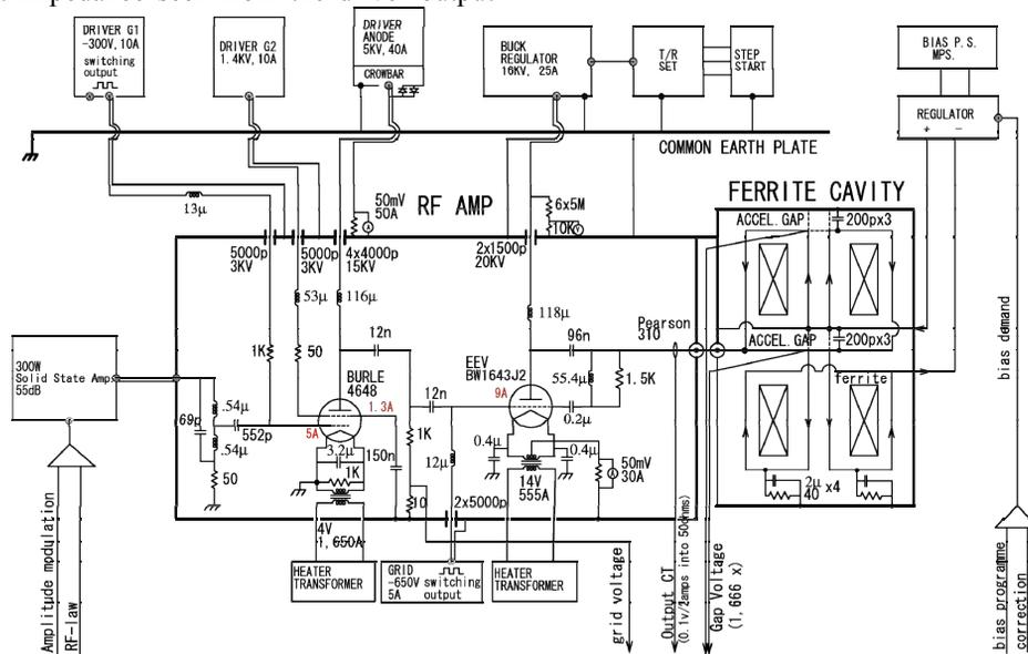
Figure 1: Layout of LOI high power drive.
