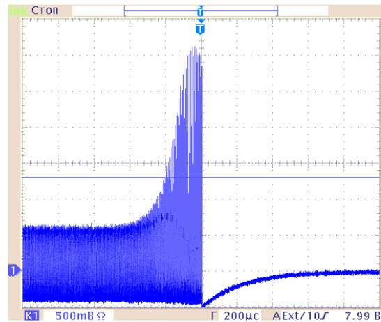
Figure 5: The bunch density increase at compression.
