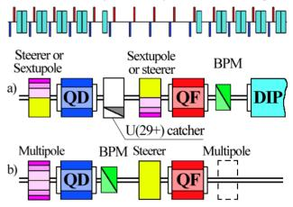
Figure 1: The SIS100 lattice superperiod and layout of the correction system units: a) in the arcs, b) in the straights.
