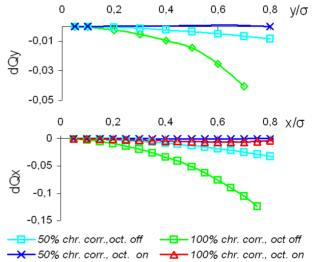
Figure 3: Amplitude dependent tune shift for the cases of 50 % and 100 % chromaticity corrections.
