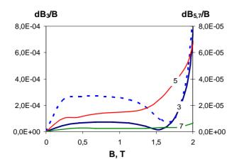
Figure 2: The systematic harmonics amplitudes of the dipole magnetic field at the radius r = 25 mm. (Dash line is the amplitude of the third harmonic in the Nuclotron dipoles).
