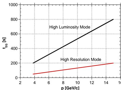
Figure 5: Cooling down times for equilibrium in HL- and HR-mode versus beam momentum.
