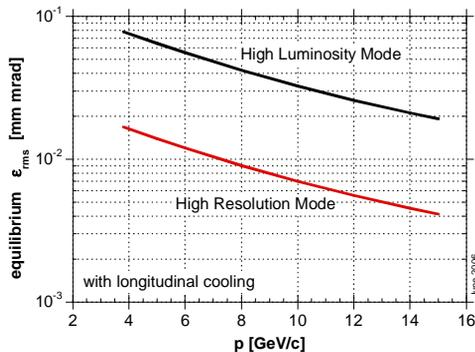
Figure 4: Transverse rms emittances versus beam momentum for the HL- and HR-mode with simultaneously longitudinal cooling.
