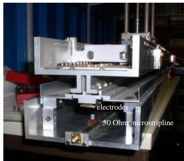
Figure 5: COSY cooling structure and test bench. The length in the beam direction reaches about 0,25m (8 electrodes).
