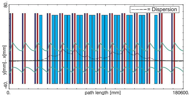
Figure 2: SIS100 lattice with the basic layout of one full sector or sextant with 14 lattice cells. The beam envelopes are shown for a beam emittance of  $e_h = 34$  mm mrad in the horizontal phase plane and  $e_v = 14$  mm mrad in the vertical phase plane respectively. The dispersion function is plotted for a momentum deviation of  $dp/p=1\%$  and the ion optical functions for the tune setting  $Q_h=18.84$  and  $Q_v=18.73$ .
