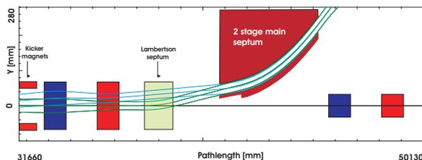
Figure 4: Detail of the extraction area. Slow (light) and fast (darker) extracted beams fit into the same aperture of the extraction septum. The depicted beams comprise twice the emittance of the extracted beam in order to define the aperture of the septa.
