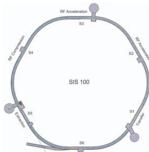
Figure 1: Distribution of the injection-, extraction-, transfer- and Rf-system (beam acceleration and bunch compression) in the six straight sections of SIS100.
