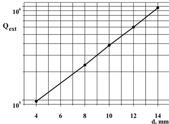
Figure 3: The Q<sub>ext</sub> dependence on gap width. ANSYS simulation data.
