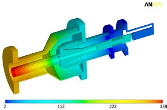
Figure 6: Temperature map of loop-capacitance coupler.
