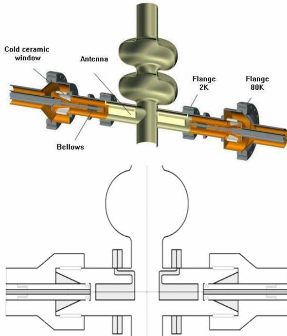
Figure 2: Coupler with capacitive element conceptual design.
