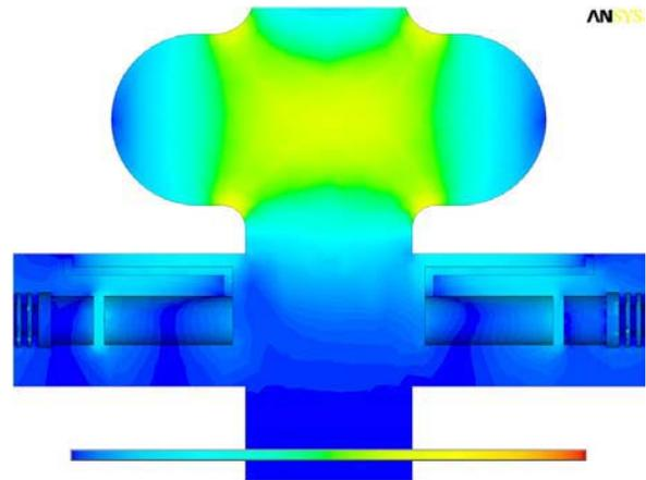
Figure 5: Antenna electric fields distribution.
