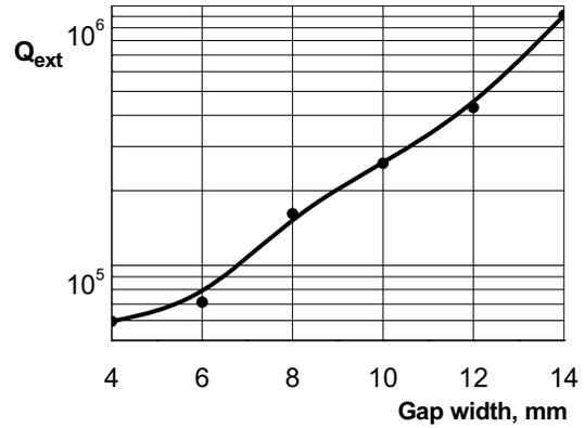
Figure 4: Dependence of Q<sub>ext</sub> of a twin coupler on the gap width. HFSS data.
