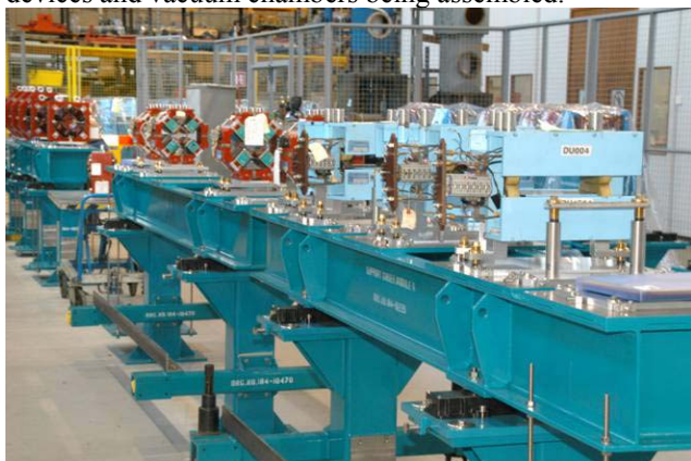
Figure 6: Modular girder assembly.
