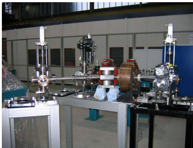
Figure 4: Gun diagnostic beamline prior to installation
