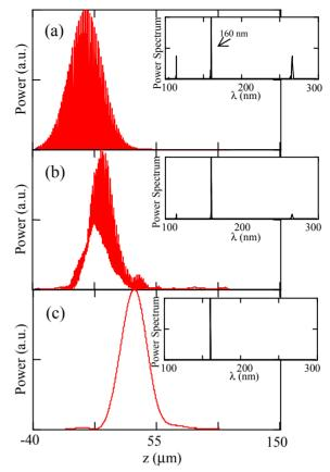
Figure 2: Power and spectrum of the radiation at different positions in the undulator for the SPARC FEL seeded at 160nm. Seed signal (a), after the first UM section (b), at the end of the undulator (c). Beam energy 200 MeV, K=1.226, the other beam parameters as in Table 1.
