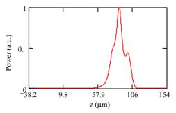
Figure 6: Longitudinal profile of the radiation power at the end of the second undulator.
