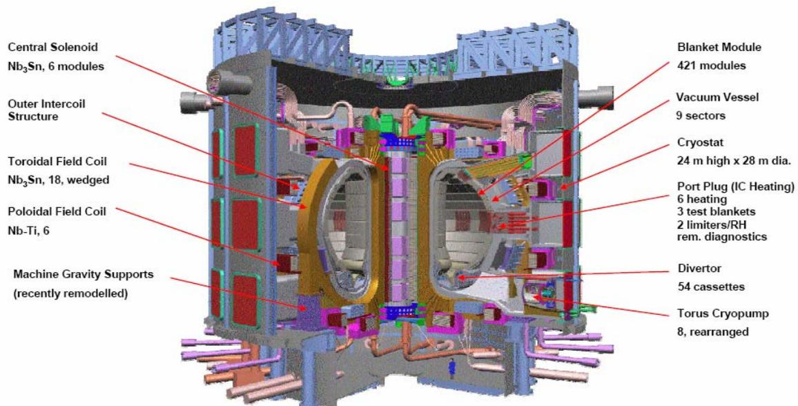
Figure 1: The ITER machine. The man in the bottom shows the scale.
