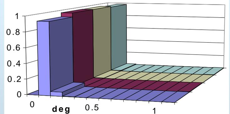
Phase error distribution recorded for 24 hours in the 4 QWRs of the PIAVE cryostat n. 1, at 5 MV/m with  $f_{1/2} \sim 3.5$  Hz
