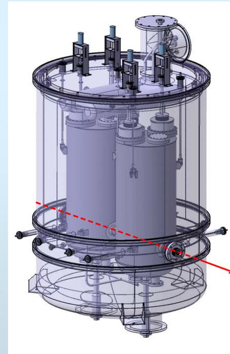
Preliminary design of the  $\beta$  0.12 cryomodule
