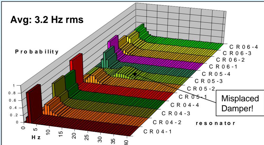
Distributions of the frequency oscillation amplitudes in a 24 hour record for all low beta cavities in ALPI.
