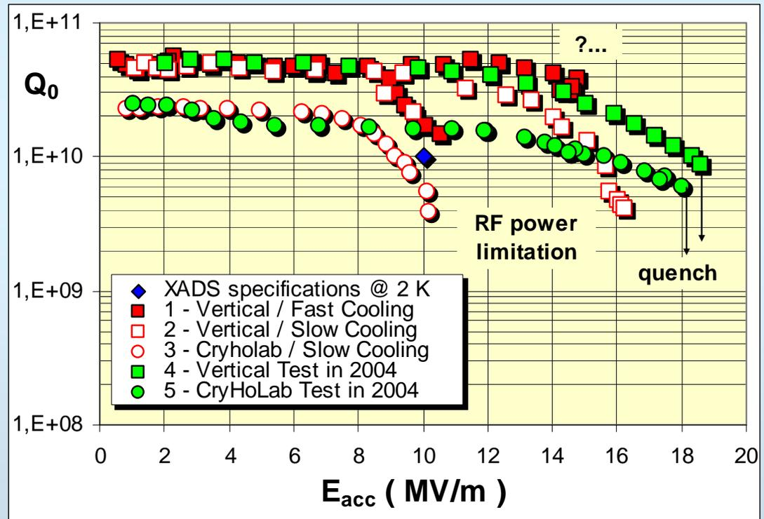
$$Q_0 = 9 \cdot 10^9 \text{ at } E_{peak} = 43 \text{ MV/m, } B_{peak} = 83 \text{ mT}$$
