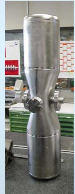
ACCEL 176 MHz SC HWR  $\beta=0.09$
