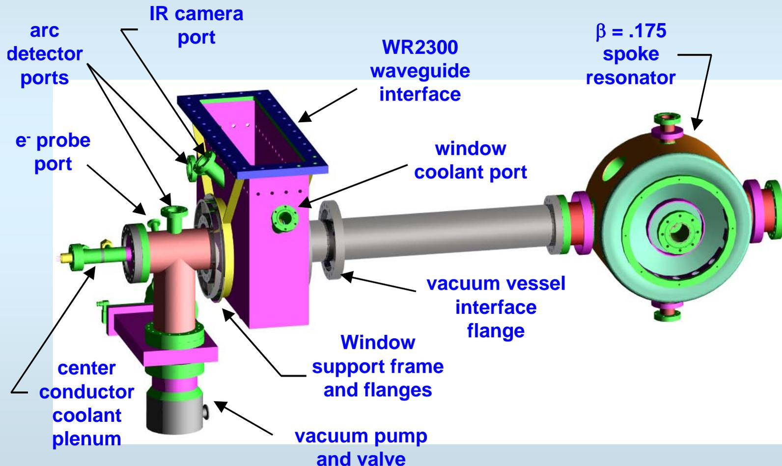
103-mm (OD) power coupler designed for up to 100 mA beam (212 kW)
