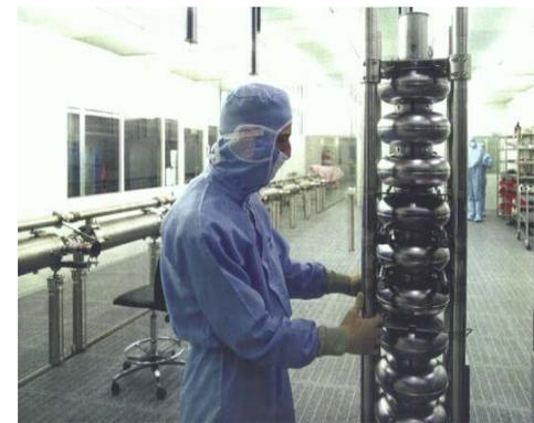
Cleanroom handling of niobium cavities
