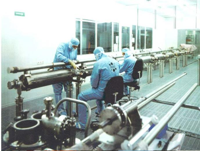
The assembly of a string of 8 cavities
