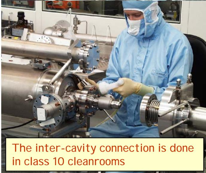
The inter-cavity connection is done in class 10 cleanrooms
