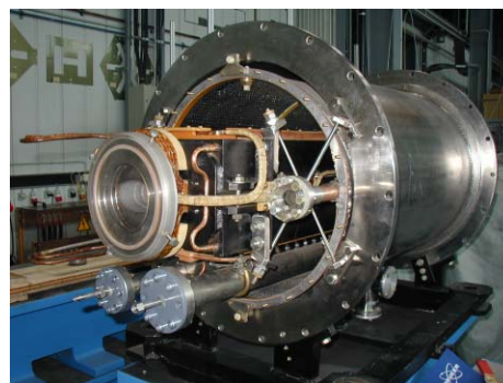
Nuclotron dipole magnet: B=2T , dB/dt=4T/s
