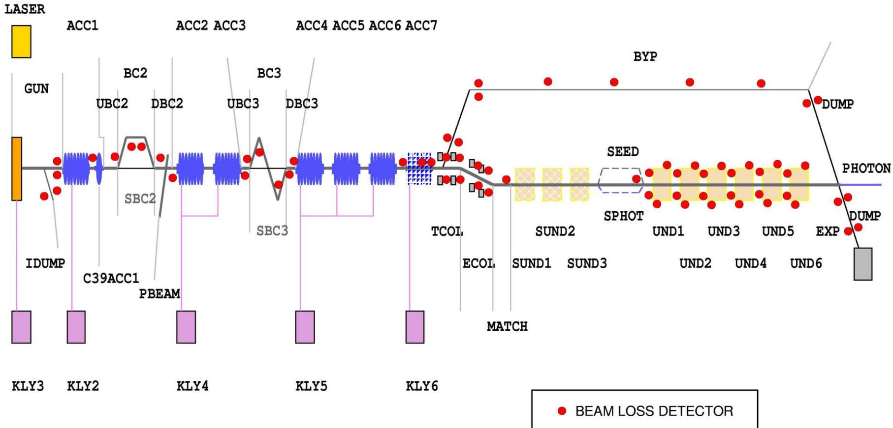
≈ 50 fast loss monitors (photomultipliers) at critical machine parts
