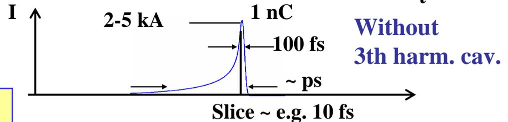
**The slice properties are relevant for the FEL process!**
