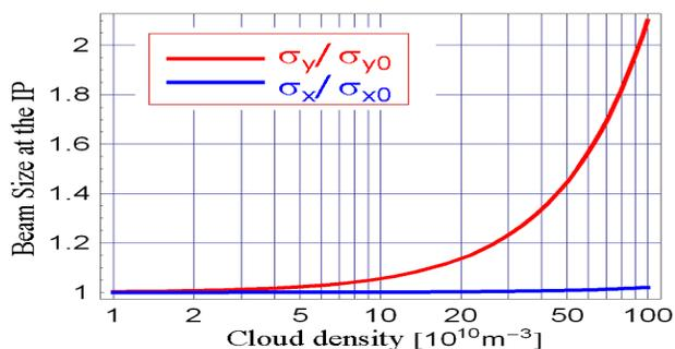
Figure 1. Simulation of beam-size blow-up at the IP as a function of the cloud density in the beam delivery system.
