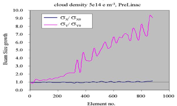
Figure 5. Beam size growth in the Prelinac section of an X-Band BCS for an above threshold cloud density  $5 \times 10^{14} \text{ e/m}^3$ .
