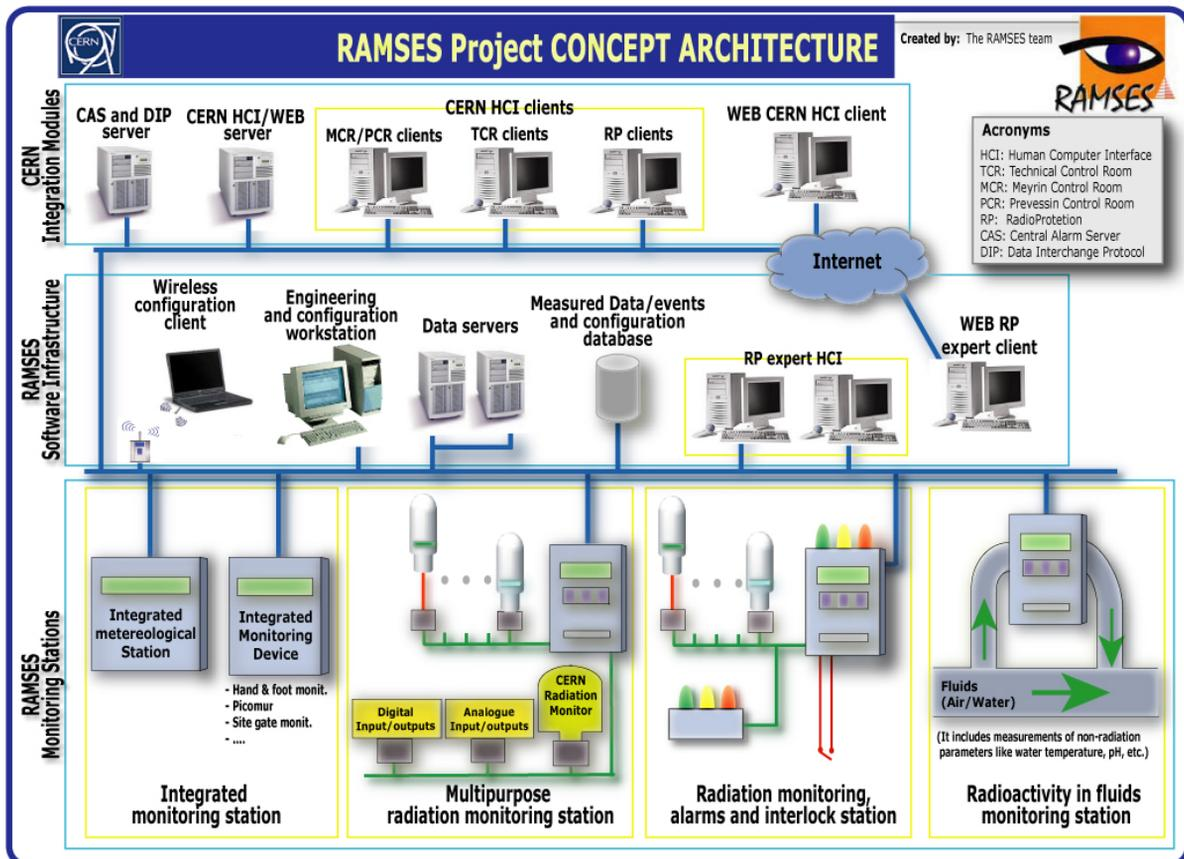
Figure 2 - RAMSES Project CONCEPT ARCHITECTURE
