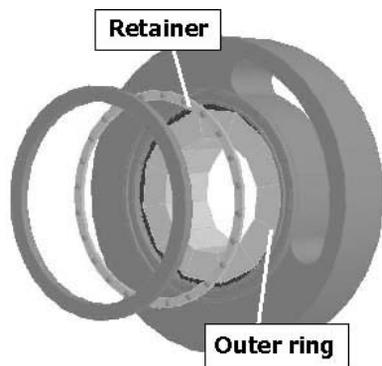
Fig. 7 Retainer with ceramic balls .
