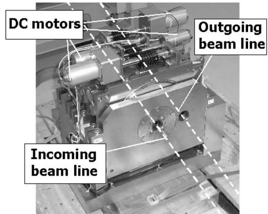
Fig. 4 Fabricated 2<sup>nd</sup> prototype PMQ
