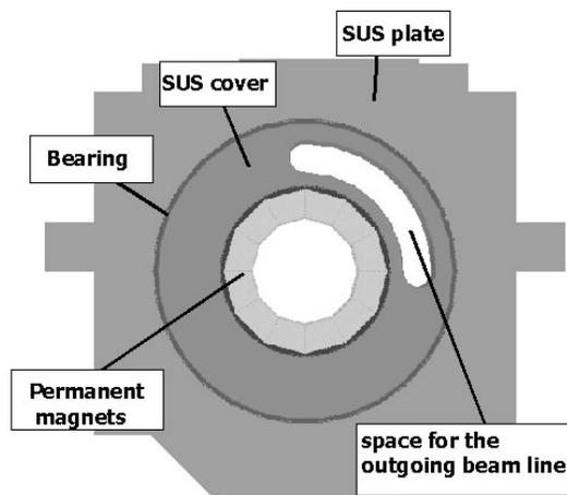
Fig. 6 Cross section showing outer ring and cover
