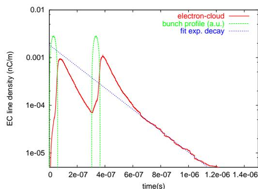
Figure 2: Line density for a field-free region of the ISIS-MW racetrack lattice.
