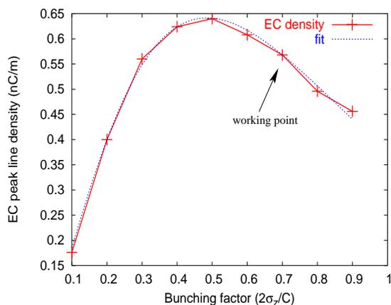
Figure 4: Variation of the peak EC line density as function of the bunching factor for the ISIS 1/2 MW upgrade scheme.
