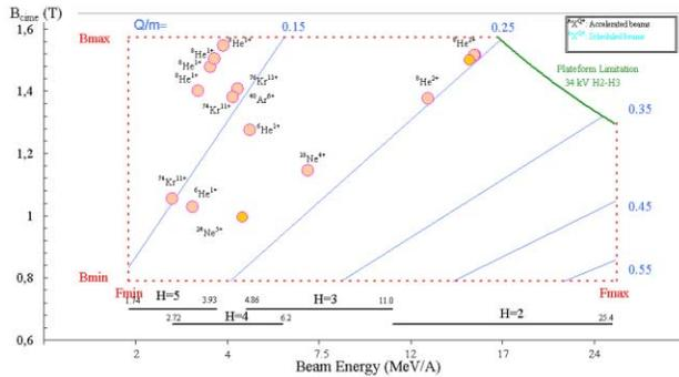
Figure 3 : CIME working diagram including accelerated beams (April 2004)
