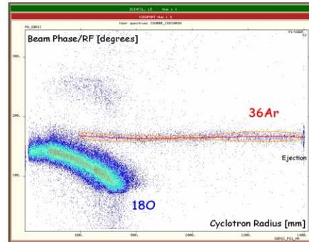
Figure 4 : Synchronism condition. Phase measurement as a function of the radius in CIME using a 300 μm silicon detector. Test realised on harmonic 3.
