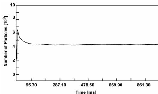
**Figure 1 :** Number of highly charged uranium ions ( $U^{73+}$ ) during acceleration in SIS18. The losses observed at the beginning of the cycle are generated by a significant life time reduction due to strong gas desorption processes.
