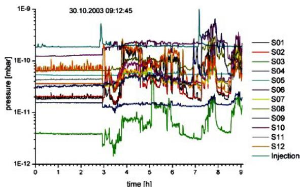
**Figure 2 :** Residual gas pressure profile in each of the twelve SIS18 sections. The initial situation (left) indicates the base pressure without beam load. The strong pressure variations (mid and right) during the beam operation phase is generated by desorbed gases from the beam pipe.
