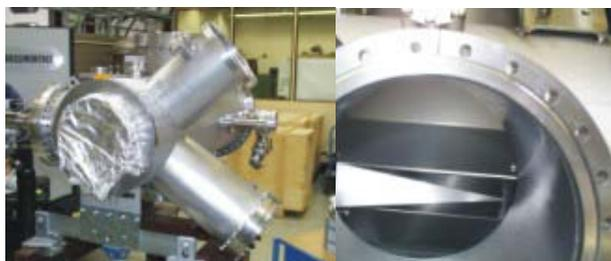
**Figure 3 :** Prototype wedge-shape desorption collimator installed in front of the electrostatic injection septum. The collimator shall protect the septum from beam losses during multi-turn injection and prevent gas desorption from the anode backside.
