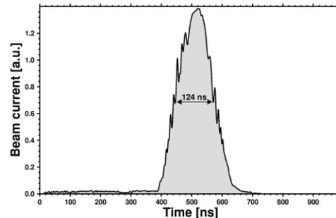
**Figure 4** : Non-linear compressed uranium bunch with  $5 \times 10^9$  ions and a FWHM length of 124 ns measured in the GSI plasma physics cave.
