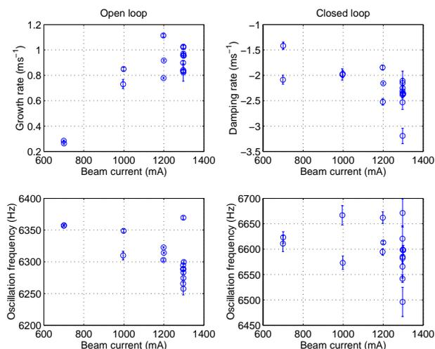
Figure 3: Open-loop growth rates and closed-loop damping rates vs. current for mode -3 in the HER.
