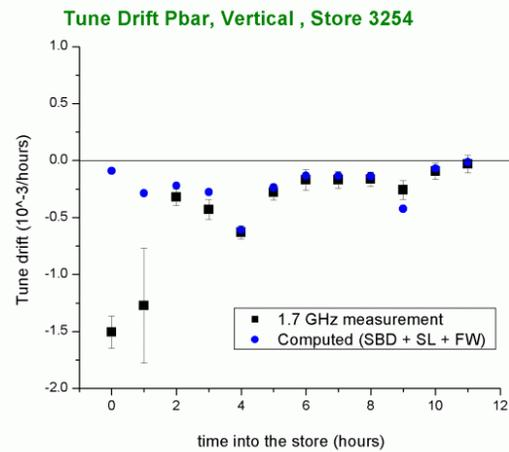
Figure 3: The antiproton tune drift during the store compared to expectation based on transverse and longitudinal emittance and intensity measurements
